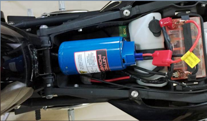
Jumpstarter in use on motorcycle. Cables store inside body and include a reverse polarity protection circuit.
